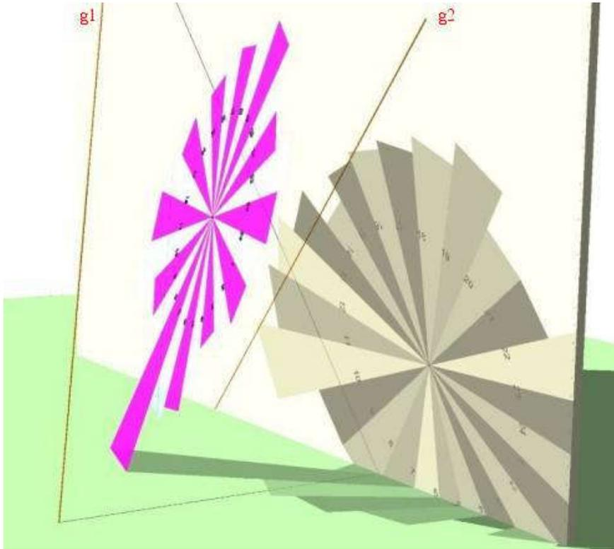
Savian separates the hour line pattern from the reading surface and places the two wires in front of, behind, or on either side of the hour line pattern. He refers to this as "positive" and "negative" wires.
