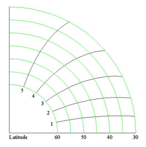
The next figure shows how to use the graph to find afternoon hour lines for a sundial for 50 degrees south.
