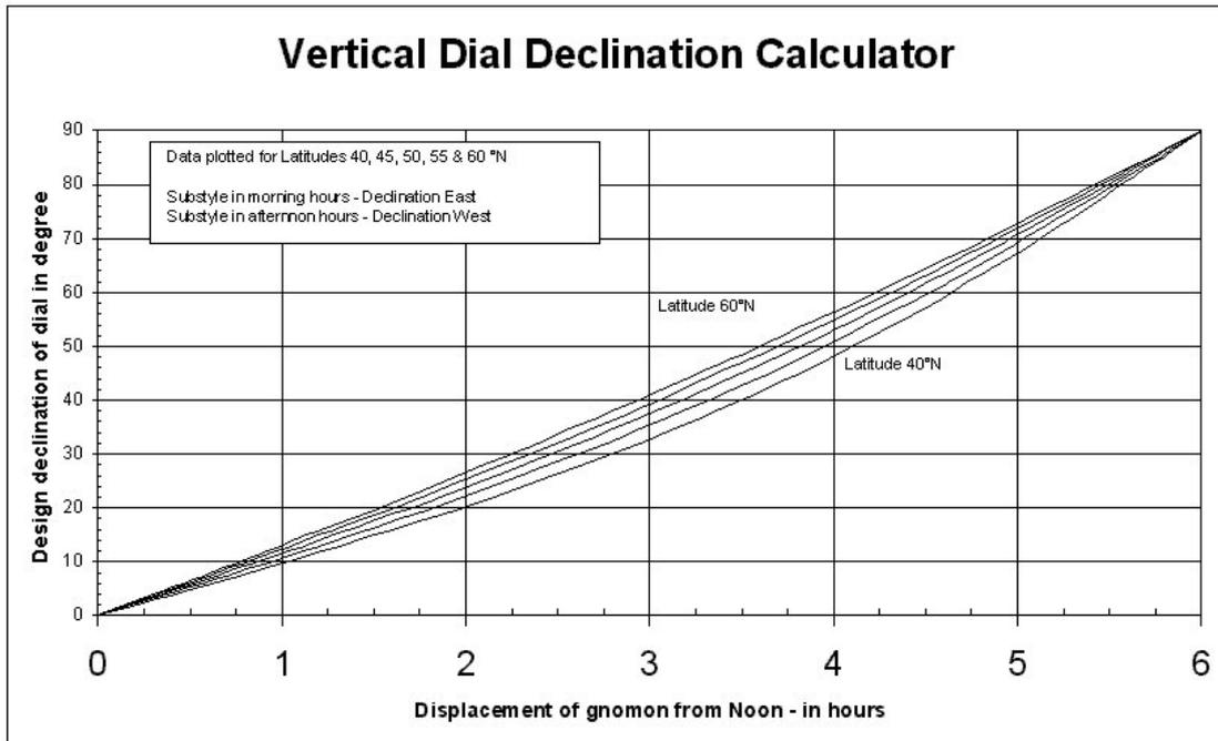
A graph of this sort makes it very easy to estimate the design declination if the position of the sub-style can be seen or inferred from the displacement in hours of the gnomon from the (local apparent) noon line.
